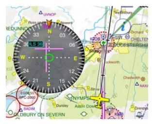
The ILS can also provide vertical guidance along a user-defined glideslope. This facility is disabled by default and needs to be manually switched on from the Navigation Options window under Setup, and an additional disclaimer agreed to. Any vertical guidance offered by the SkyDemon ILS should always be compared to your cockpit instruments. Regardless, the vertical guidance will cancel when you descend through 500ft above aerodrome level.
