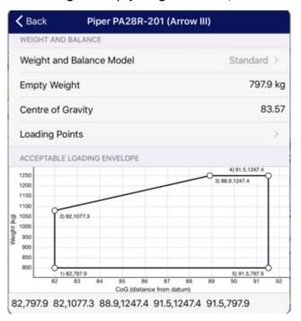
about each of the loading points applicable. A loading point is just a place in the aircraft where weight is applied, whether fuel, passengers, baggage or anything else. These are usually provided in the POH or a balance sheet accompanying the aircraft. When you create a new aircraft profile we
