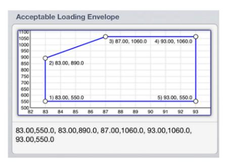
actual centre of gravity and total weight of the aircraft is calculated, the value is plotted on the graph. If it falls within the polygon, the aircraft is safely configured.
