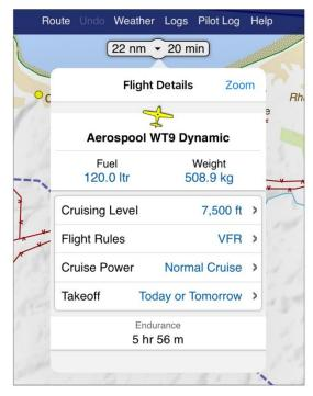
To change the cruise speed for your route click Cruise Power in Flight Details and select a power setting from the list.
