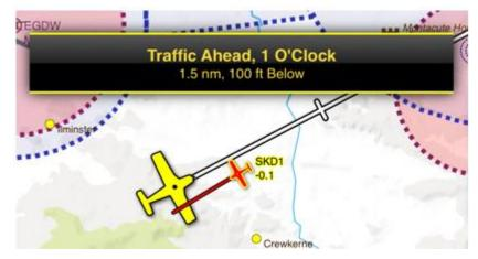
Next to each aircraft symbol you will see a number, a plus (+) or minus (-) symbol and an arrow pointing up or down. This number represents the aircraft's relative altitude, with a + to indicate that it is above you or a - if it's below, and an up or a down arrow to show if it is climbing or descending. If it's level you won't see an arrow.
