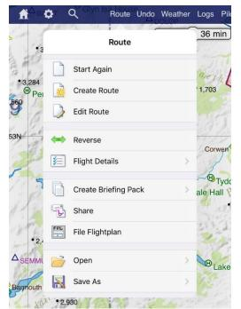
Routes can be saved in GPX and RTE formats, a couple of Garmin flightplan formats, and even in KML format for viewing the magenta line in Google Earth as a 3D fly-through.
